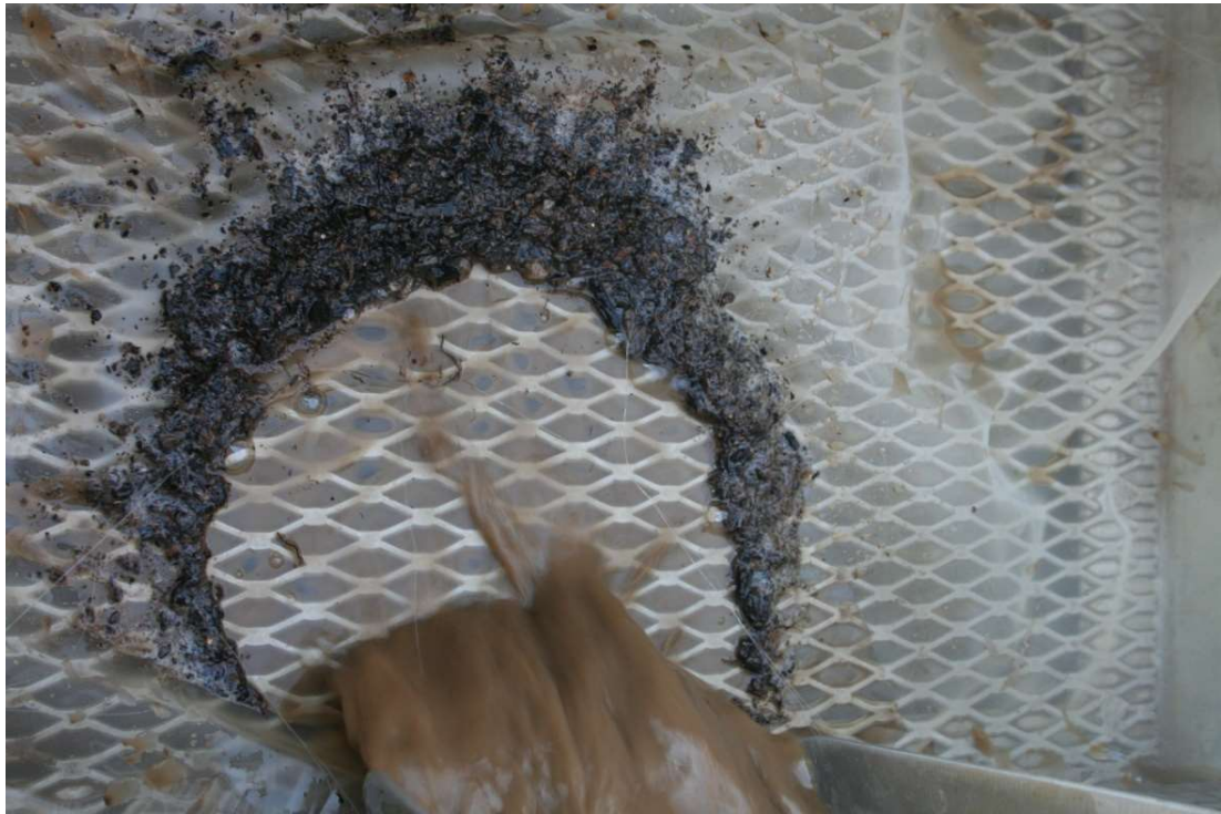
Figure 04: Light fraction recovery in 0.325 mm fine mesh.
