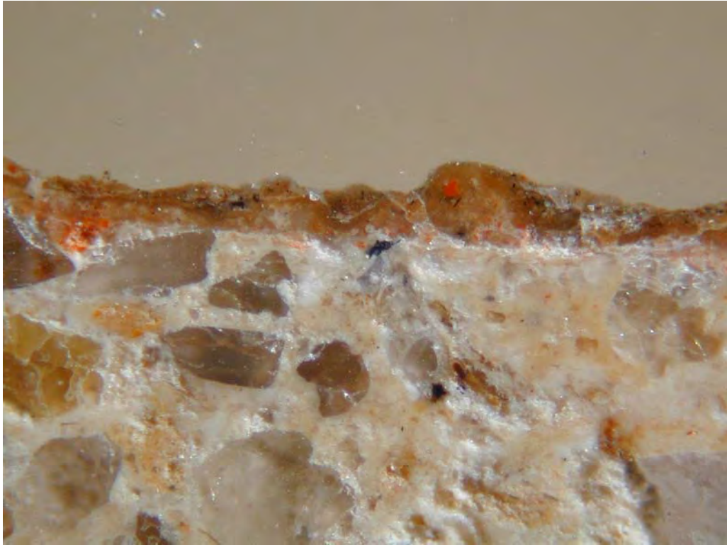
Photomicrograph attached to email “ Jamestown house 5 mortar sample,” Mark Kutney to Carl Lounsbury, 4 April 2002 showing what appear to be a pigmented coating on the mortar.
